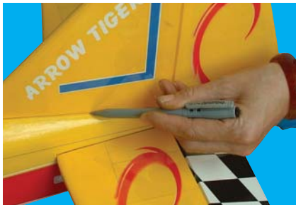
11B- Mark both sides of the vertical stabilizer
