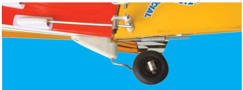
24A - The rudder pushrod is connected to the rudder control horn
