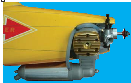
18A- Fuel line connected to the carburetor and pressure line connected to the muffler.
