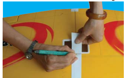
3C- Trim off the excess tape.
