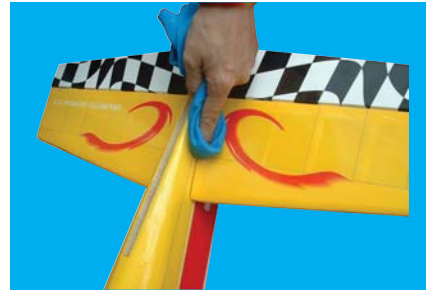
10D- Wipe off excess epoxy
