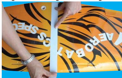
3B- Continue applying the tape over the bottom of the wing, pressing down firmly as you go.
