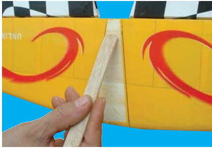
10B- Apply plenty of epoxy
