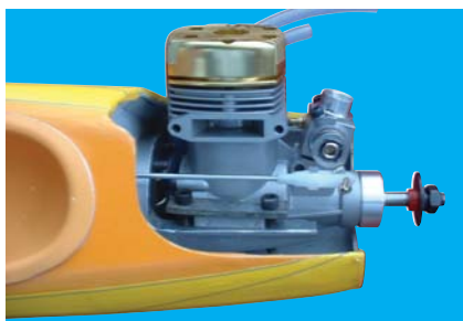
17A- Clevis attached to engine throttle arm
