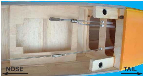
22B- Pre-installed elevator, throttle and rudder pushrod
