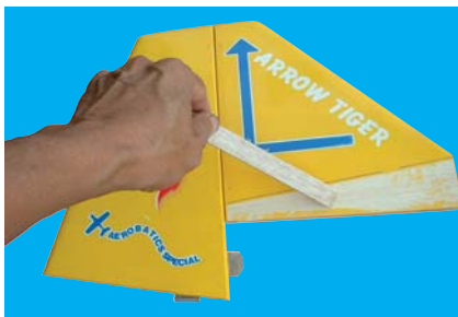
12A- Apply plenty of epoxy
