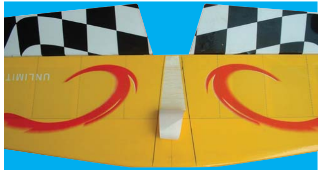
9C- Remove the covering from top surface.
