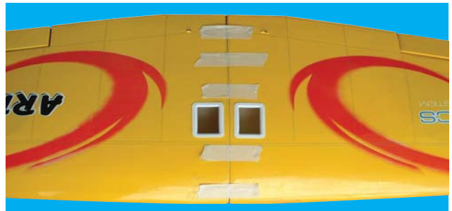
2C- Use low tack masking tape to hold tightly together.
