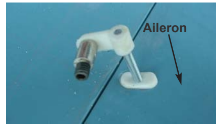
4E- Install aileron control horn
