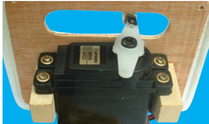
4D- Screw servo in position
