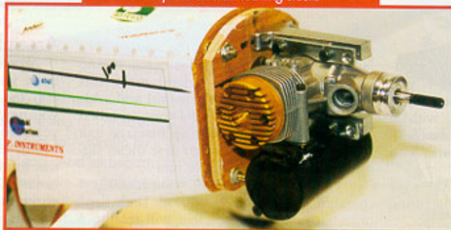
Below: The engine is mounted onto the supplied engine mount and an in-cowl muffler is used to keep the aircraft looking sleek.
