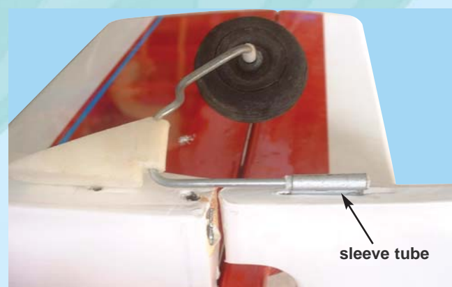
15B - Insert the tail wheel components into the pre-installed sleeve tube
