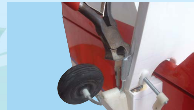
15D - Trim off the excess tail steering wire
