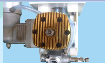
19A - Fuel line connected to the carburetor and pressure line connected to the muffler
