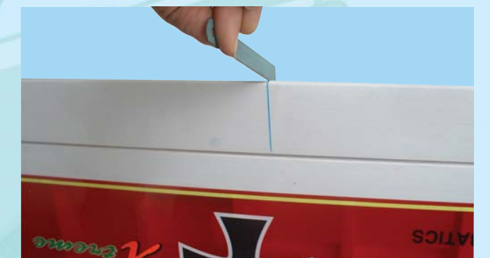
34B - Using the hack saw blade to cut quad flap mark
