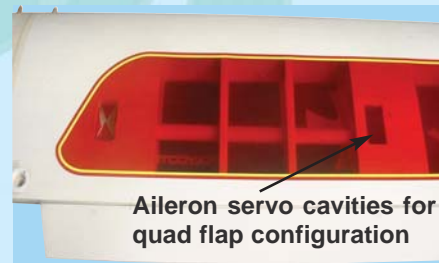
4C - Aileron servo cavities for quad flap configuration. (See Stage 34)
