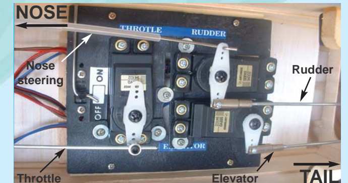
22C - Throttle, rudder and elevator servos connected to their push rods as referenced left to right
