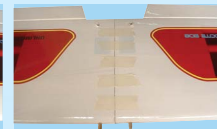
2C - Use low tack masking tape to hold tightly together
