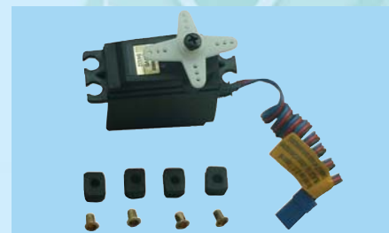
4A - Prepare the servo by fitting the rubber grommets & ferrules supplied with your radio
