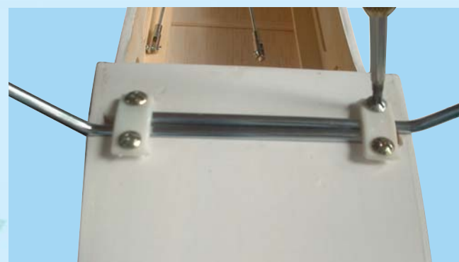
14D - Use 4 sheet metal screws and 2 straps to mount the main landing gear onto the fuselage
