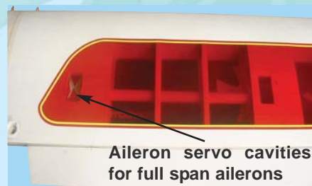
4B - Aileron servo cavities for full span ailerons
