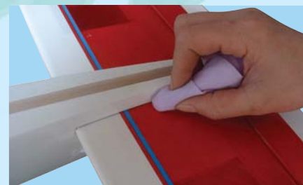
10D - Wipe off excess epoxy
