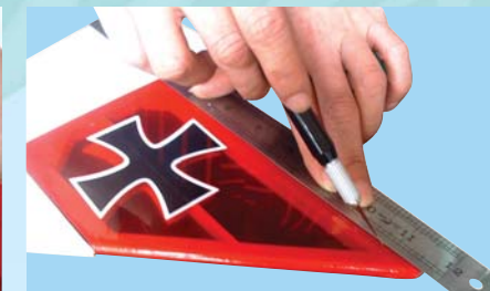
11C - Carefully cut through the covering. DO NOT CUT THE WOOD
