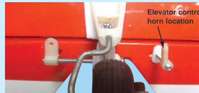
21C - Elevator control horn location
