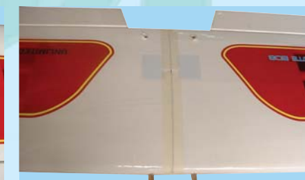
3C- Continue over to the bottom of the wing & along to the servo cavity and trim off the excess tape
