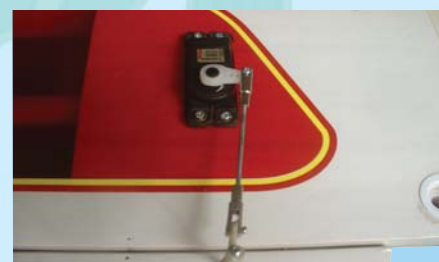
5C - Aileron servo and control rod installed
