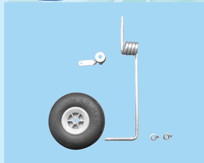
15A - Nose gear components
