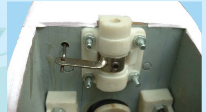
15D - Place the steering arm into the slot in the nylon nose gear bearing
