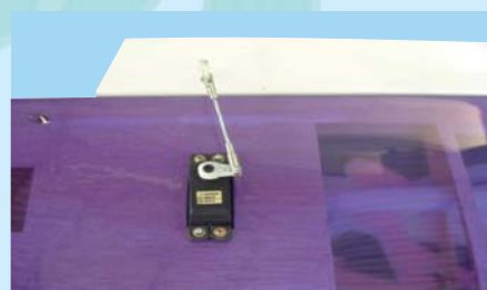
5C - Aileron servo and control rod installed
