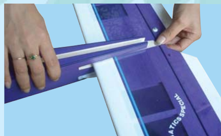
10C - Slide the horizontal stabilizer in place
