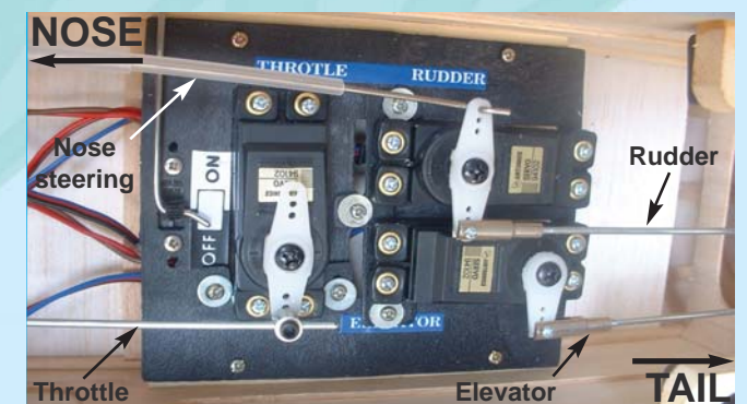
22C - Throttle, rudder and elevator servos connected to their push rods as referenced left to right
