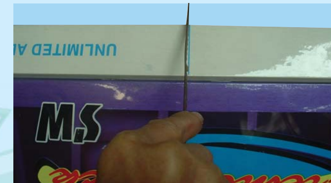
35A - Use a hack saw blade or a hobby razor saw to cut through the ailerons at the locations marked
