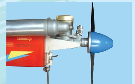
20A - The spinner and propeller attached to the engine
