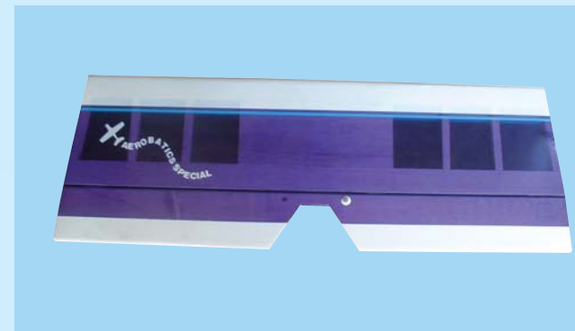
6B - Horizontal stabilizer with pre-installed elevator
