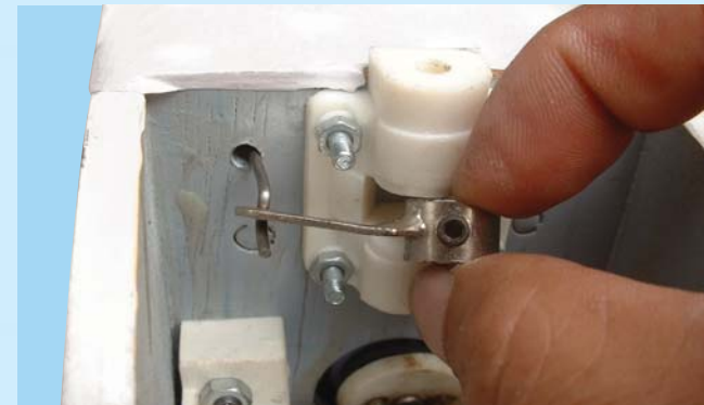
15C - Insert the end of the pre-installed Z-bend wire into the hole in the steering arm
