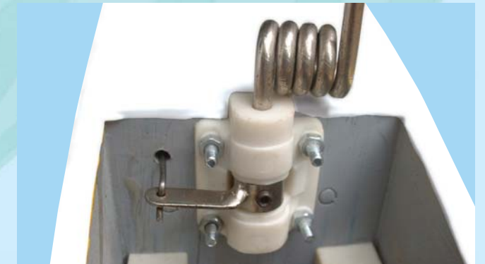
15F - Typical nose gear installation when complete
