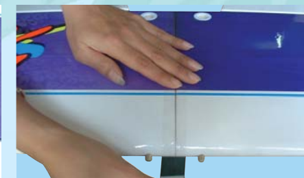
3B- Continue applying the tape over the top of the wing, pressing down firmly as you go
