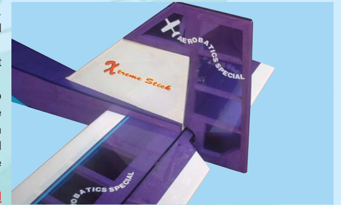
11A - Trial fit the vertical stabilizer into fuselage slot.
