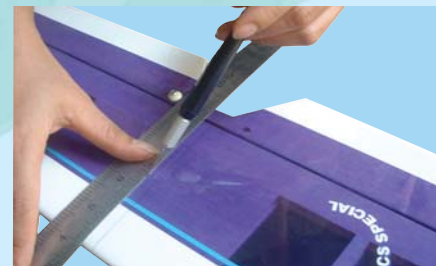
9B - Cutting inside the lines. DO NOT CUT THE WOOD
