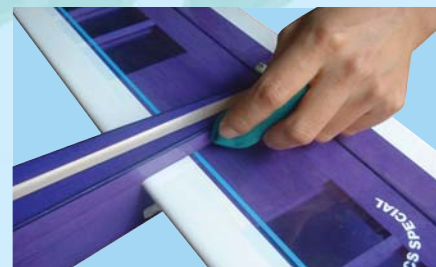
10D - Wipe off excess epoxy
