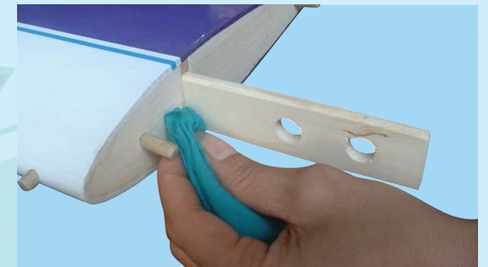
1F - Wipe off the excess epoxy then allow to cure
