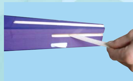
10A - Apply plenty of epoxy
