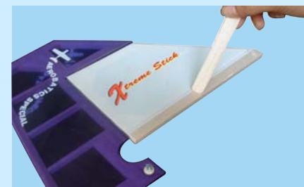
12A - Apply plenty of epoxy
