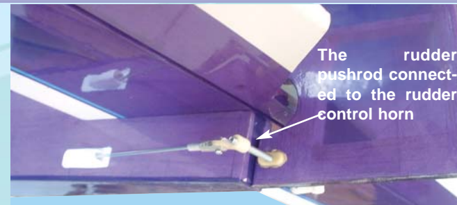
25A - The rudder pushrod connected to the rudder control horn
