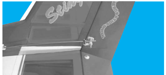
25A. The rudder pushrod is connected to the rudder control horn
