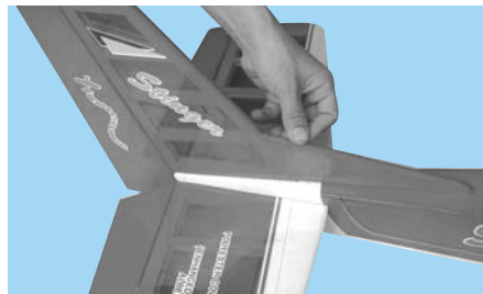
12B. Slide the stab into place & remove excess epoxy
