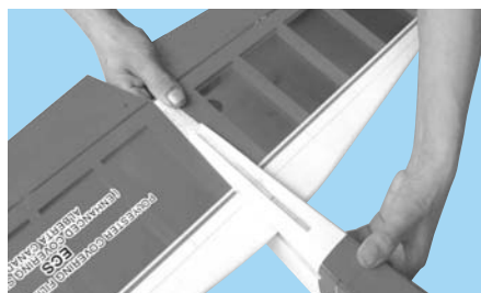
10C. Slide the horizontal stabilizer in place
