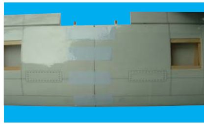
2D - Use tape to hold tightly together
