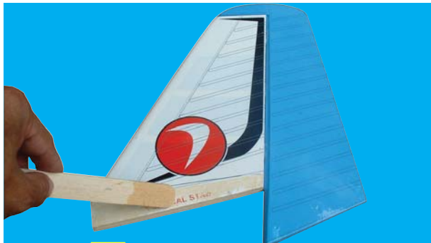
14A - Apply plenty of epoxy
