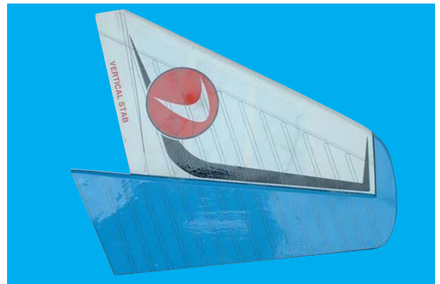
7C - Vertical stabilizer with pre-installed rudder
