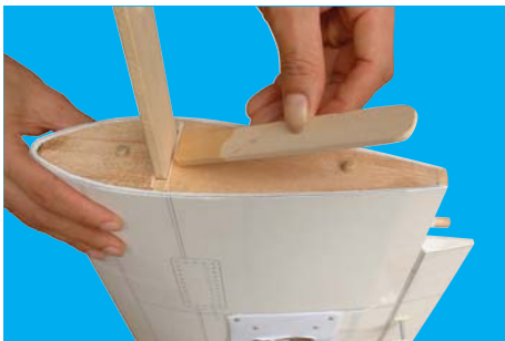
2A - Apply plenty of 30 minute epoxy glue to all surfaces.
