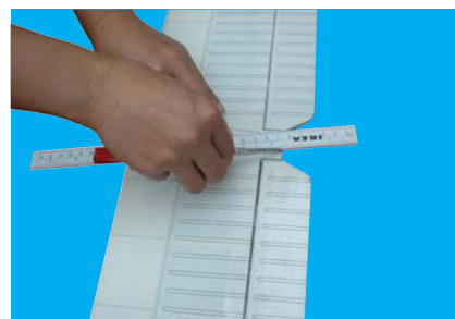
10B - Cut 1/8" inside the lines
