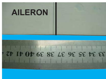
6B - Mark a line at 14-3/4" (375mm) from the wing-tip using a water soluble non-permanent felt-tip pen
