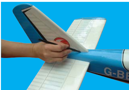
13A - Mark both sides of the vertical stabilizer
