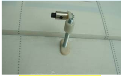
6E - Install the control horn assembly to the flap
