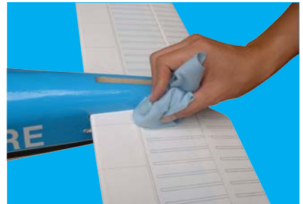
11C Wipe off excess epoxy
