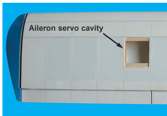
4B - Aileron servo location
