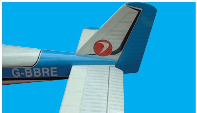
12A - Trial fit the vertical stabilizer into fuselage slot.
