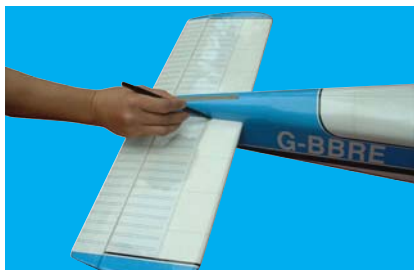
9A Mark the top of the horizontal stabilizer ...
