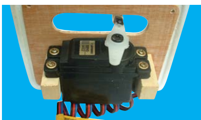
4D - Screw servo in position
