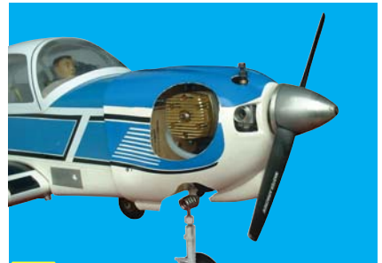
19C - Install suitable Propeller and spinner after finishing the cowl installation.
