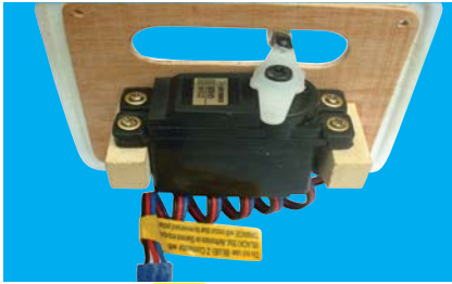
6D - Install flap servo to the servo mount
