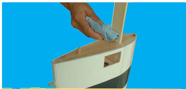
1F - Wipe off the excess epoxy then allow to cure.
