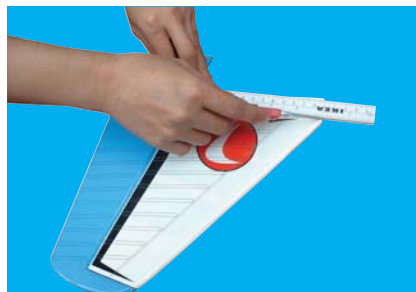
13B - Carefully cut through the covering... NOT into the wood.
