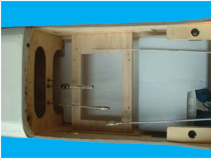
22B - Pre-installed elevator, throttle and rudder pushrod
