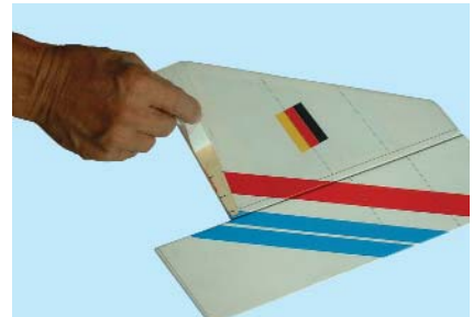
11.3 Remove covering from both sides
