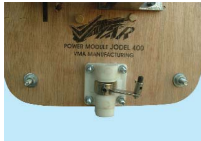
14.1 Insert the EZ connector threaded shaft through the steering arm, secure with a nut and place the arm into the nylon nose gear bearing
