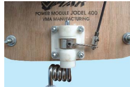
14.5 Loosen the EZ connector bolt to adjust the movement of the nose gear
