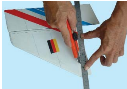
11.2 Carefully cut through the covering
