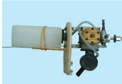
17.6 Engine and fuel tank in position on the power module
