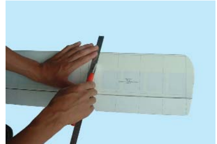
8.2 Cutting inside the lines
