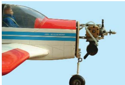
17.12 Power module mounted to the fuselage (side view)
