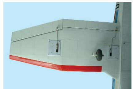
4.4 Final flap installation
