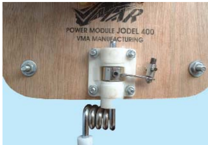
14.3 Holding the nose gear steering arm in place, slide the nose gear into the nylon mount, passing through the steering arm.
