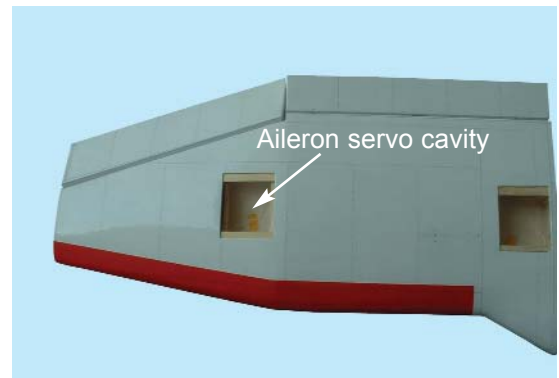
2.2 Aileron servo location
