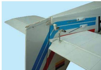
22.1 Rudder control horn installed and shown in position
