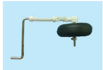
15.3 Main landing gear assembly
