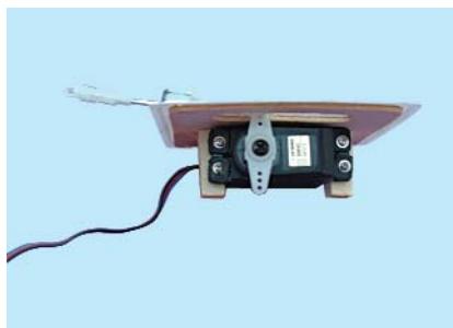
4.3 Flap servo in position
