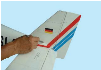
11.1 Mark both sides of the vertical stabilizer
