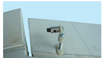
2.5 Install aileron control horn
