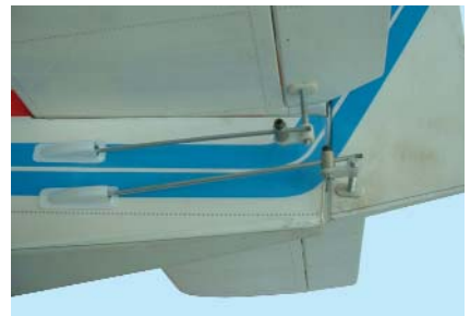
22.2 Connecting the rudder pushrod to the rudder control horn
