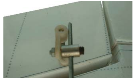
3.3 Aileron control installed
