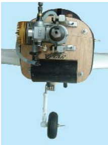
17.11 Power module mounted to the fuselage
