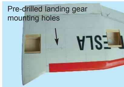
15.2 Main landing gear location
