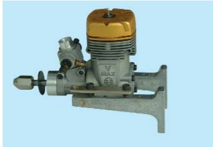
17.5 Fitting the engine to the engine mount
