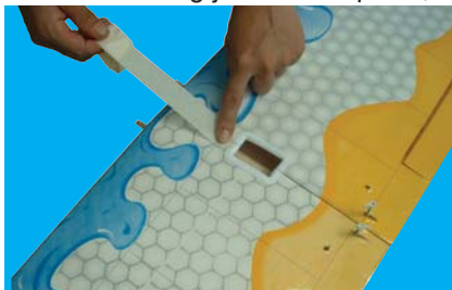
3A- Apply tape over the joint, starting here
