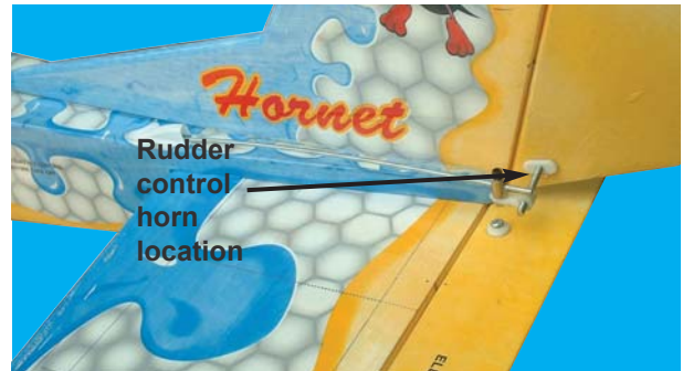
21D- Rudder control horn location
