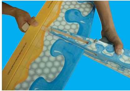
10C- Slide the horizontal stabilizer in place
