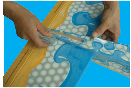
10D- Wipe off excess epoxy
