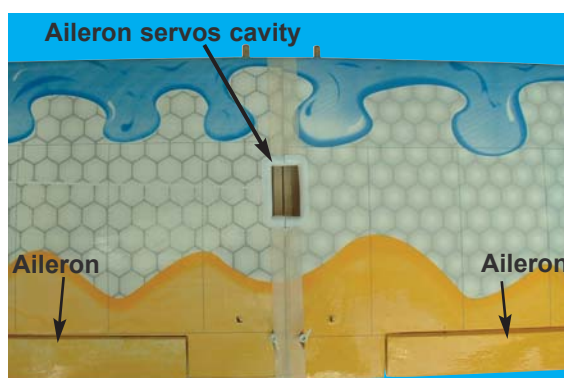
4B- Aileron servo location
