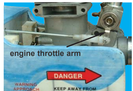
26B- Throttle control rod connected to the engine throttle arm
