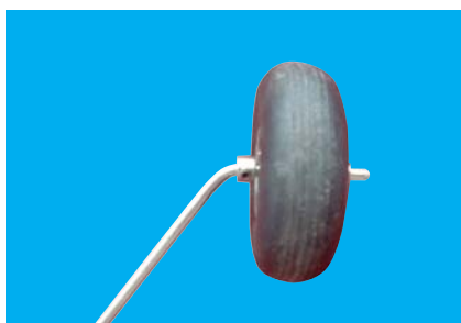
14B- Installation of collars and wheel to the pre-bent main landing gear wire.
