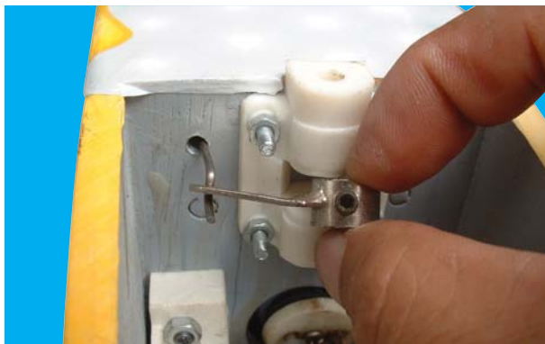
15C- Insert the end of the pre-installed Z-bend wire into the hole in the steering arm
