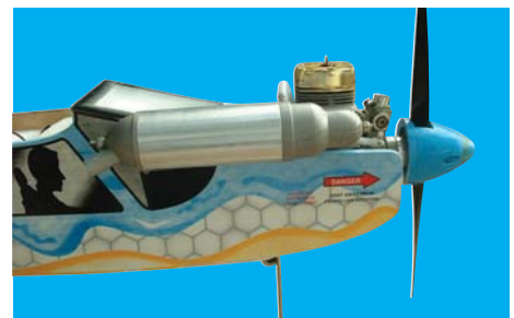
20A- The spinner and propeller attached to the engine.
