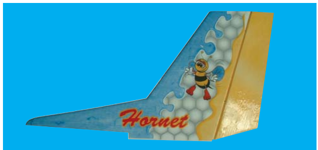
6C- Vertical stabilizer with pre-installed rudder
