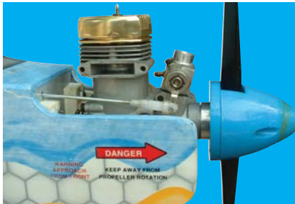
18A- Clevis attached to engine throttle arm
