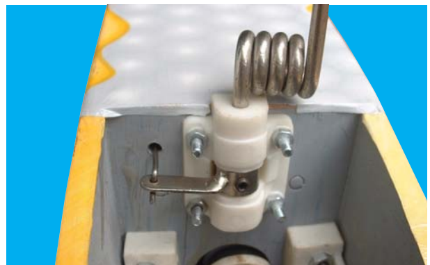
15F- Typical nose gear installation when complete.
