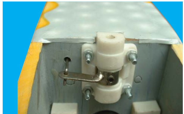
15D- Place the steering arm into the slot in the nylon nose gear bearing
