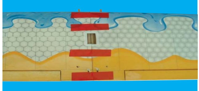
2C- Use low tack masking tape to hold tightly together.
