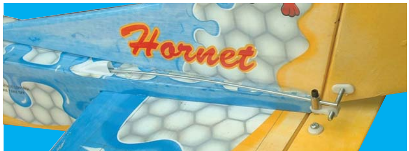
25A - The rudder pushrod is connected to the rudder control horn
