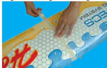
3B- Continue applying the tape over the top of the wing, pressing down firmly as you go.
