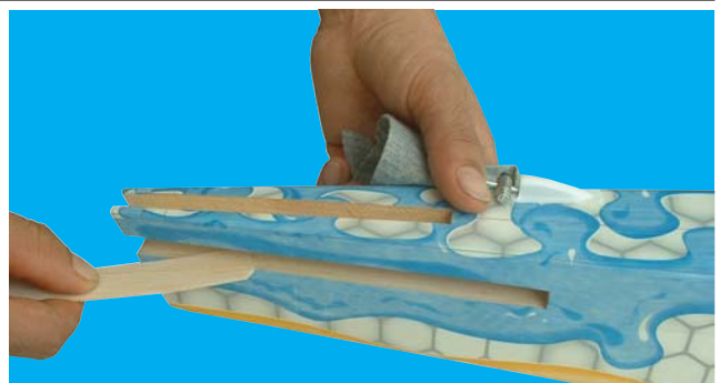
10A- Apply plenty of epoxy
