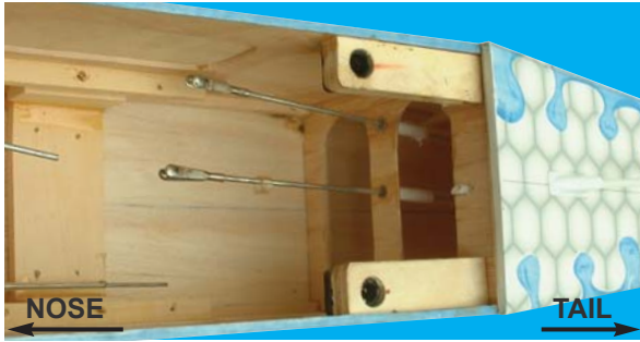
23B- Pre-installed elevator, throttle and rudder pushrod
