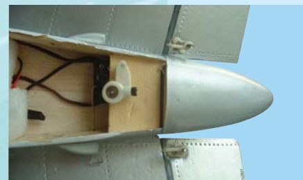
16D - Rudder control horn installed
