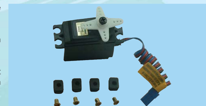
2A - Prepare the servos by fitting the rubber grommets & ferrules supplied with your servos
