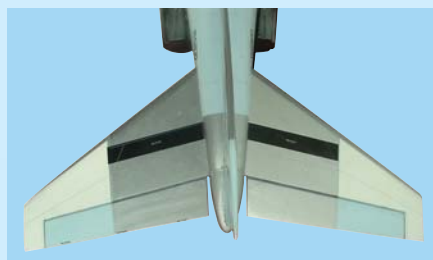
6B - Trial fit the horizontal stabilizers into the fuselage slots
