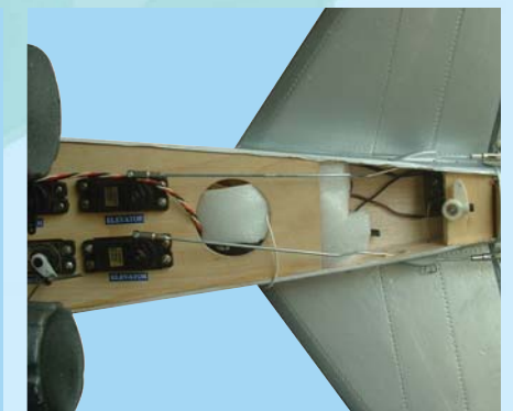
19B - Install the rudder control horn to the rudder control arm
