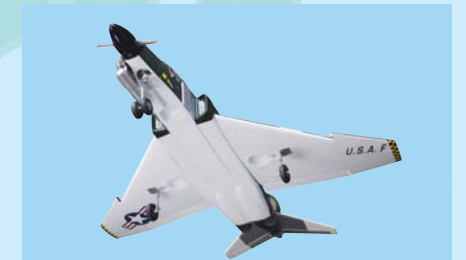
8D - Main landing gear mounted to both wings
