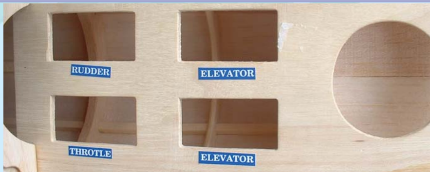
17A - Location of elevator (2), rudder and throttle servos
