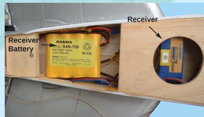
24B - Receiver battery and receiver location
