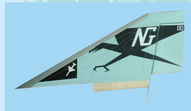
4B - Vertical stabilizer with pre-installed rudder
