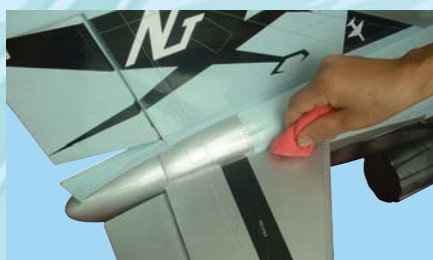
6E - Wipe off the excess epoxy
