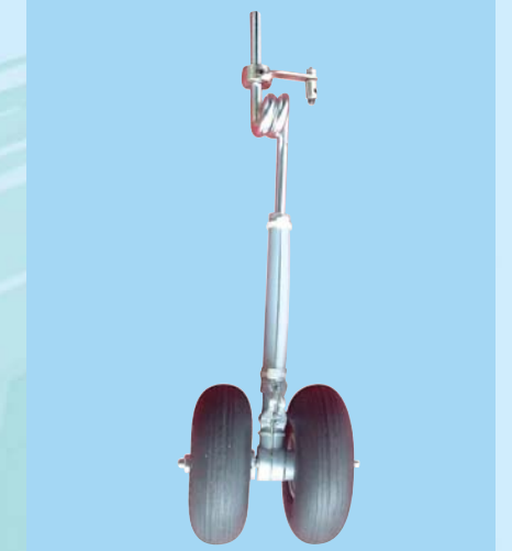
9A - Nose gear assembly
