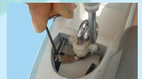
9D - Secure the EZ-connector to the nose gear push rod by tightening the set screw
