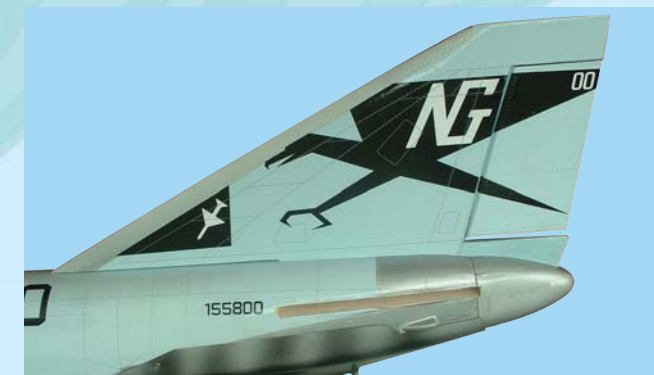
5C - Trial fit the vertical stabilizer in its slot
