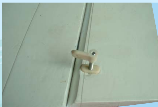
3B - Aileron control horn installed
