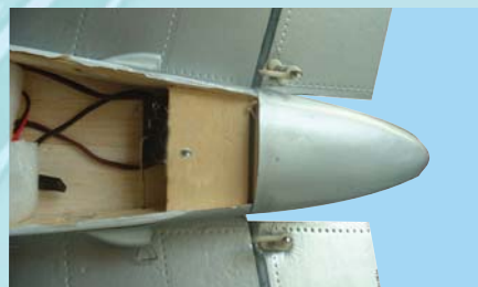
16C - Elevator control horns installed
