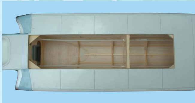
1B - Bottom hatch cover removed
