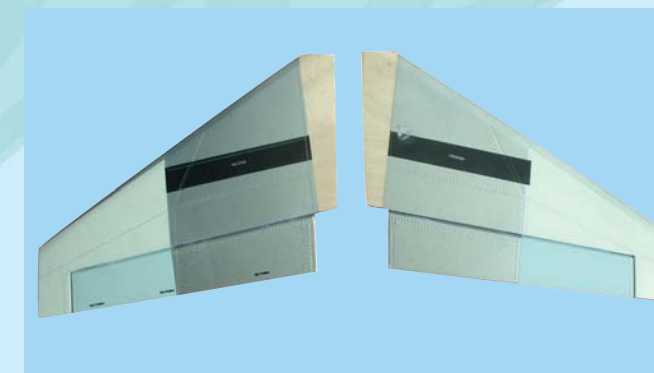
4C - Horizontal stabilizer with pre-installed elevators
