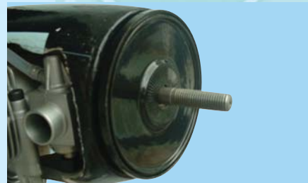
15B - Install the spinner backing plate
