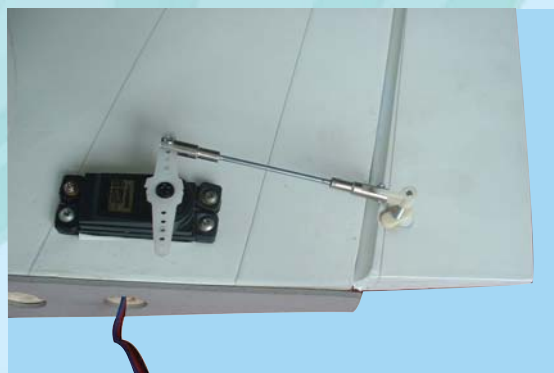
3C- Aileron control rod installed
