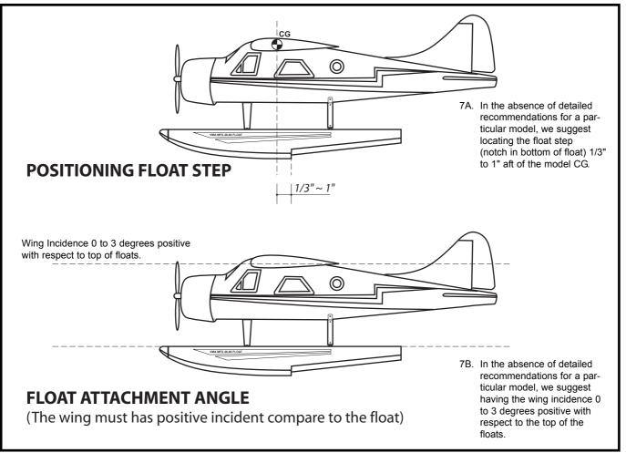
7A. In the absence of detailed recommendations for a particular model, we suggest locating the float step (notch in bottom of float) 1/3" to 1" aft of the model CG.
