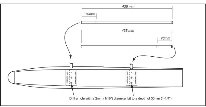
1B. Insert the 2 aluminum spreaders into the left float
