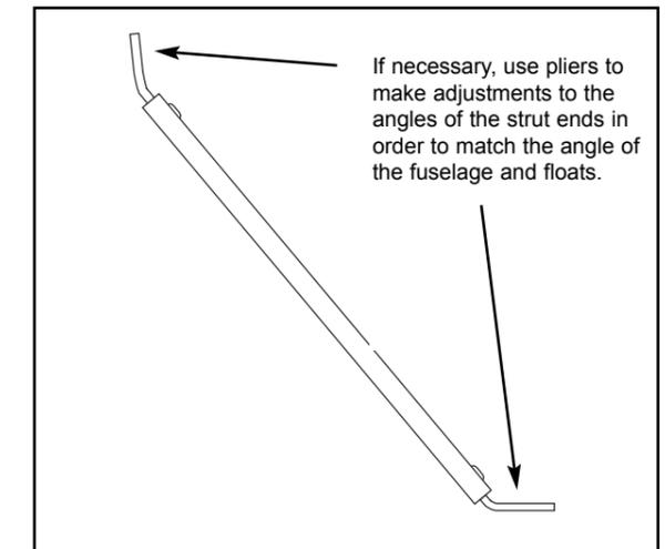
If necessary, use pliers to make adjustments to the angles of the strut ends in order to match the angle of the fuselage and floats.
