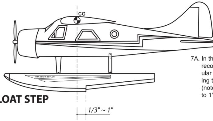
7A. In the absence of detailed recommendations for a particular model, we suggest locating the float step (notch in bottom of float) 1/3" to 1" aft of the model CG.
