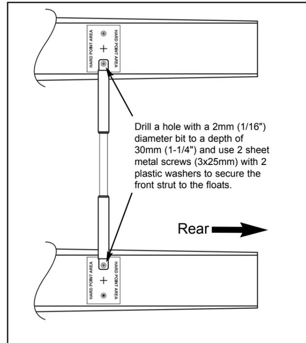
Drill a hole with a 2mm (1/16") diameter bit to a depth of 30mm (1-1/4") and use 2 sheet metal screws (3x25mm) with 2 plastic washers to secure the front strut to the floats.
