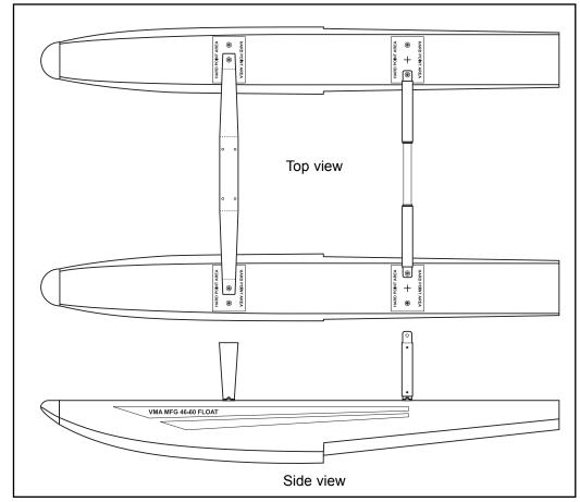
4C. Top and Side view of floats with struts attached.
