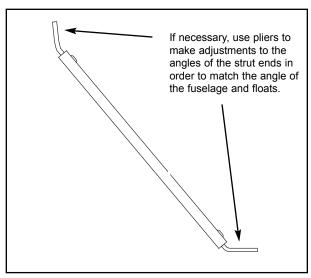
4B. Adjust the angles of the rear strut ends.
