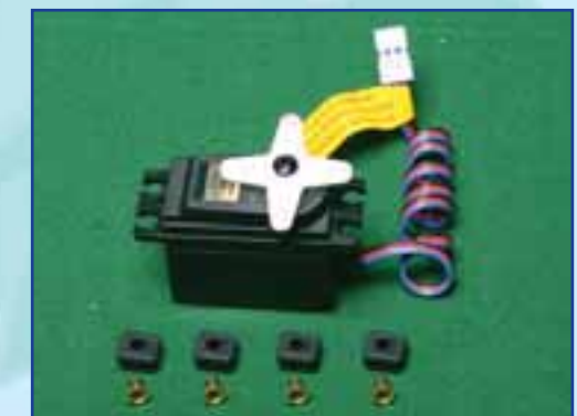
2A. Prepare the servos by fitting the rubber grommets & ferrules supplied with your radio
