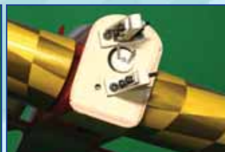
14D. Install the fuel tank into the fuselage. Seal neck area with silicone.
