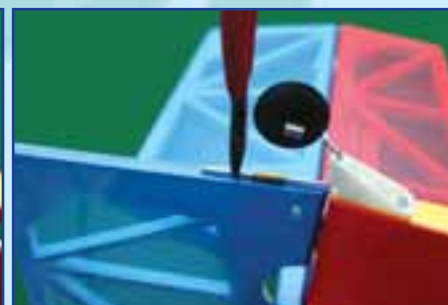
13C. Trim off the excess tail wheel steering wire with side cutters.
