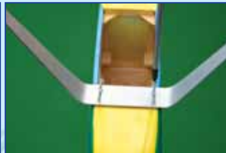
12D. Use 4 metal sheet screws (5 x 35mm) to mount the main landing gear onto the fuselage
