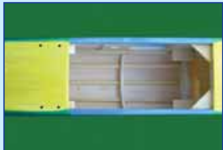
12C. Locate the 4 pre-drilled main landing gear mounting holes on the bottom of the fuselage.
