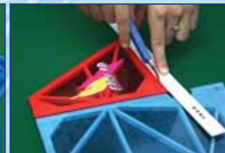
10B. Carefully cut through the covering. Do NOT cut into the wood.
